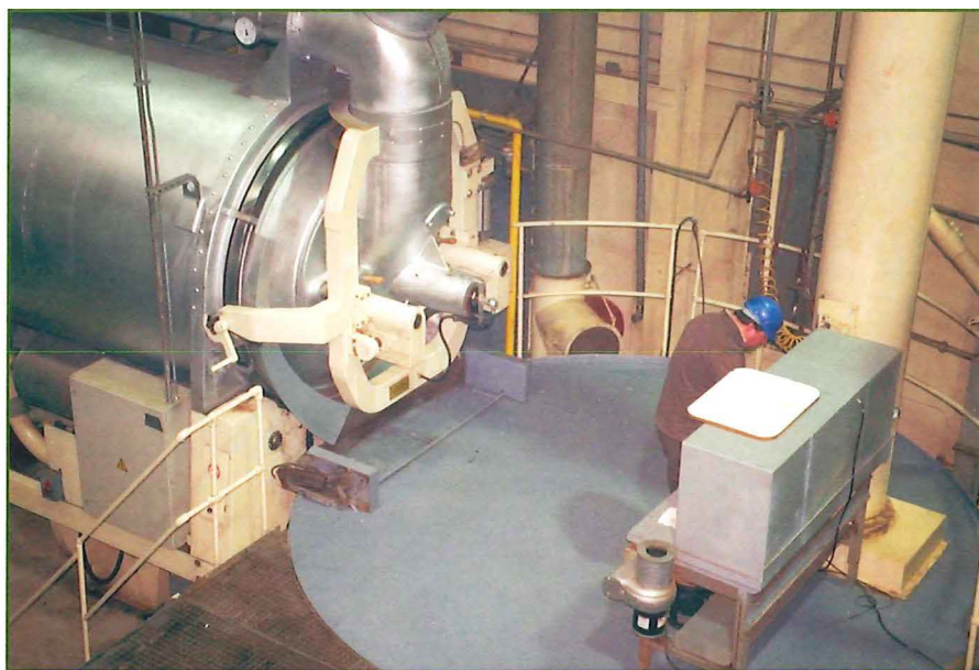
Briess drum roaster used for making specialty malts.
